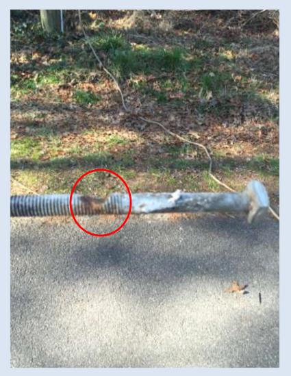
This bolt was arcing to a bracket. Note the bolt is 50% eroded.
